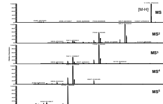
Figure 9 – Irganox 1010 APCI Negative Ion Mass Spectrum, MS n on 0.22 ng on-column
