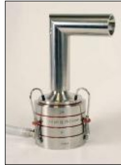
Copley Short-Stack Fast Screening Andersen Impactor (C-FSA) used in TMI studies
