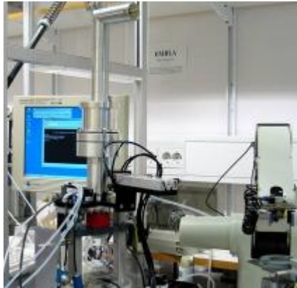
AstraZeneca Fully-Automated Single Cut-Off Stage Impactor (SSI) (see Lundbäck and Wiktorsson RDD-2006; 467-470 for semi-automated version)
