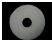
Liquid EtOH deposits on stage '0' of full ACI
